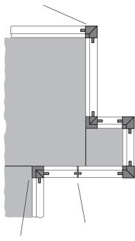
Connecting wedge Inner corner conector
